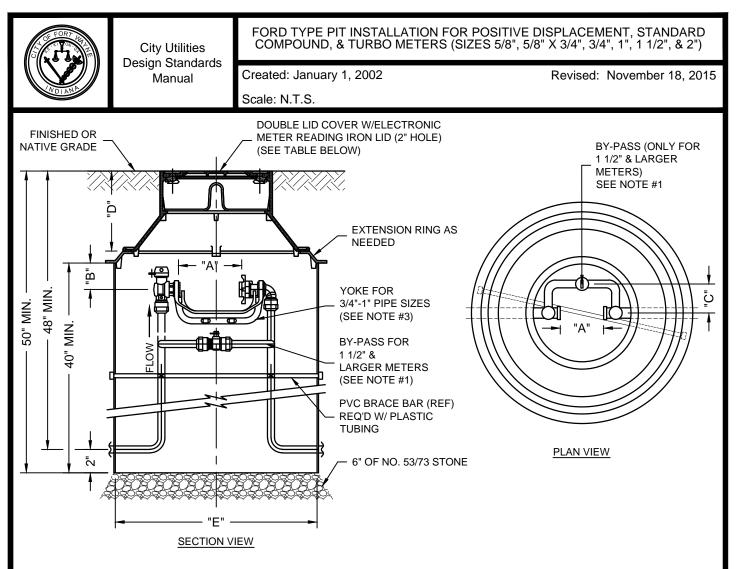
"A" = SPACE REQUIRED FOR METER FROM FACE OF FLANGES OR FOR METER YOKE
