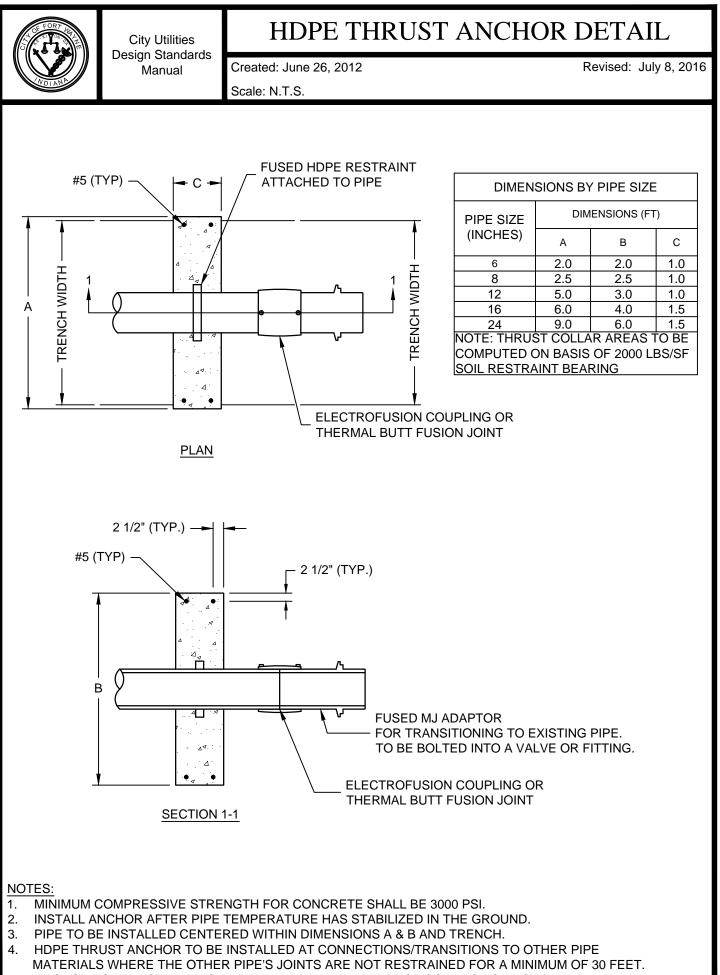
5. ANCHOR TO BE INSTALLED ON HDPE MAIN WITHIN 25 FEET OF CONNECTION POINT.
