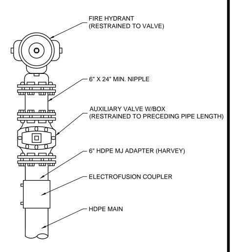
FIRE HYDRANT ASSEMBLY TYPE V- HDPE
