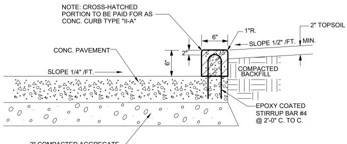
2" COMPACTED AGGREGATE-#53 FOR BASE ON APPROVED SUBGRADE
